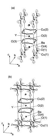
FIG. 2. Structure of YBa<sub>2</sub>Cu<sub>3</sub>O<sub>7-x</sub>. (a) The orthorhombic *Pmmm* phase. (b) The tetragonal *P4/mmm* phase. Note that in the tetragonal phase the oxygen atoms are disordered in the z = 0 plane.
