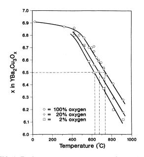
FIG. 6. Total oxygen content vs temperature for samples of  $YBa_2Cu_3O_{7-x}$  heated in flowing 100% O<sub>2</sub>, 20% O<sub>2</sub>-80% Ar, and 2% O<sub>2</sub>-98% Ar atmospheres. At each oxygen partial pressure the orthorhombic-to-tetragonal transition occurs near a stoichiometry of  $YBa_2Cu_3O_{6.5}$ .
