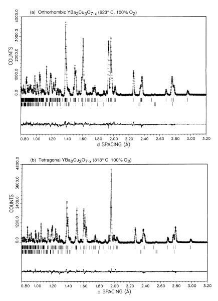
FIG. 1. Rietveld refinement profiles for (a) orthorhombic  $YBa_2Cu_3O_{7-x}$  at 623 °C and (b) tetragonal  $YBa_2Cu_3O_{7-x}$  at 818 °C. Plus marks (+) are the raw neutron powder diffraction data and the continuous line is the calculated profile. Tick marks below the curves indicate the positions of the allowed  $YBa_2Cu_3O_{7-x}$  reflections (upper tick marks) and a minor CuO impurity phase (lower tick marks) included in the refinements.
