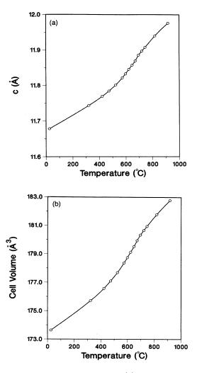
FIG. 5. The c-axis lattice parameter (a) and unit-cell volume (b) vs temperatures for YBa<sub>2</sub>Cu<sub>3</sub>O<sub>7-x</sub> in 100% oxygen.
