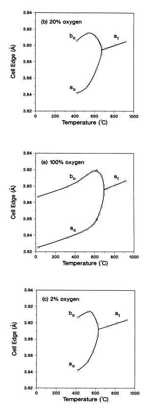
FIG. 4. The *a*- and *b*-axis lattice parameters of YBa<sub>2</sub>Cu<sub>3</sub>- $O_{7-x}$  vs temperature for samples heated in (a) 100% O<sub>2</sub>, (b) 20% O<sub>2</sub>-80% Ar, and (c) 2% O<sub>2</sub>-98% Ar.
