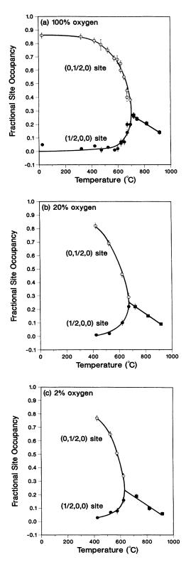
FIG. 7. Fractional oxygen site occupancies at the indicated sites in YBa<sub>2</sub>Cu<sub>3</sub>O<sub>7-x</sub> vs temperature for a sample heated in (a) 100% oxygen, (b) 20% oxygen, and (c) 2% oxygen. Since the allowed occupancy for the  $(\frac{1}{2}, 0, 0)$  site in the tetragonal phase is two atoms per unit cell, the fractional occupancies for this site must be doubled to yield the number of oxygen atoms per unit cell.
