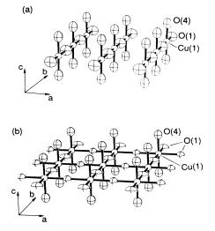
FIG. 3. Detail of the oxygen-atom ordering in the z = 0 plane of YBa<sub>2</sub>Cu<sub>3</sub>O<sub>7-x</sub>: (a) Orthorhombic phase exhibiting complete ordering of oxygen atoms onto the  $(0, \frac{1}{2}, 0)$  site which results in one-dimensional CuO<sub>3</sub> chains along the *b* axis; and (b) tetragonal phase showing a disordering of the oxygen atoms in the same plane.
